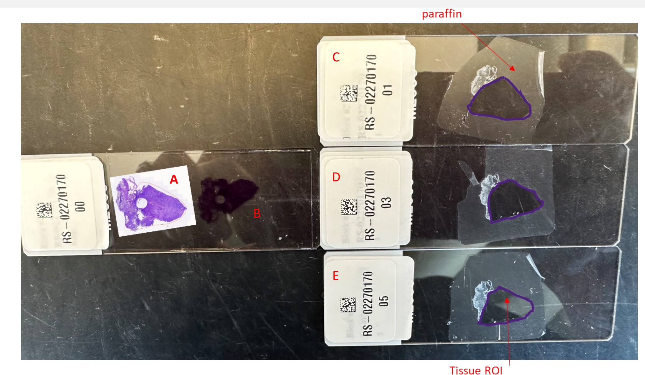
Figure 4. Case RS-02270170. A) H&E image with ROI marked red. B) H&E slide. C - E) Images of replicate unstained slides with tissue scraped and removed by Tissector HT in marked ROI.
